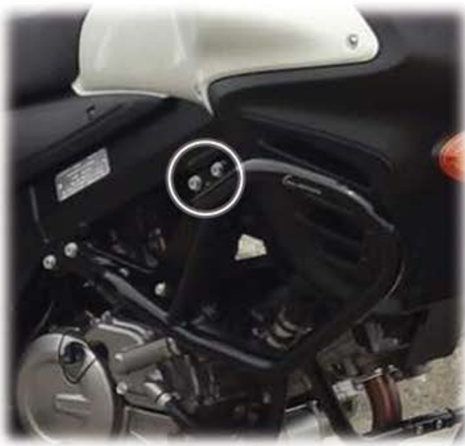
REMOVE THE ORIGINAL SCREWS
