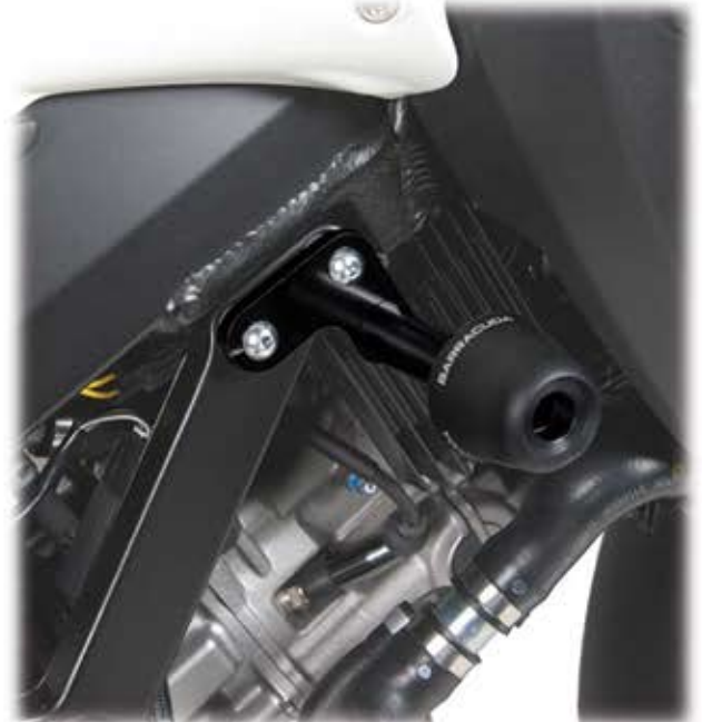
INSTALL THE KIT SAVE CARTER USING THE THICKNESS BETWEEN THE CHASSIS AND THE SPECIFIC BRACKET
