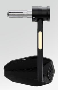
Two mirrors must always be fitted, as indicators are integrated.
