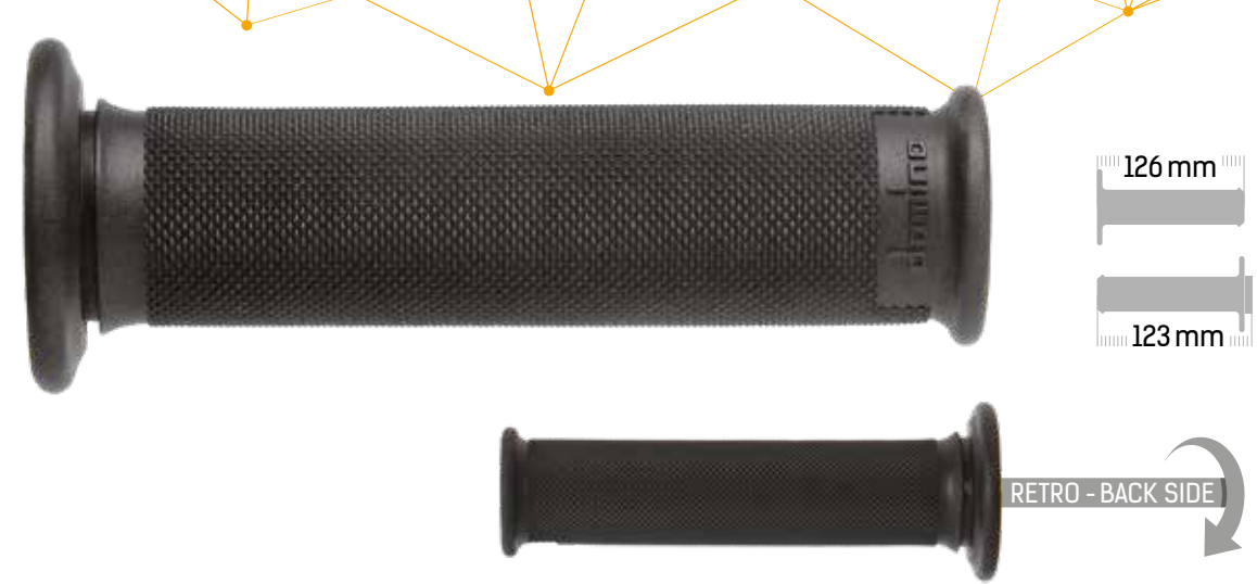
6280 | cod. 6280.82.40 Nero - Black Manopole monocolore in gomma termoplastica Monochrome grips in rubber compound
