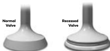
Figure: Common Valve Recession in a Natural Gas Engine
