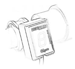
Insert the Glpro unit into the housing, pushing it firmly to the back to ensure good adhesion. If you ever need to remove the Glpro from the housing, use a small flat head screwdriver to lift it up. Do NOT pull the cable!
