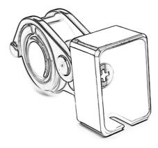
Place the housing in the desired orientation and fasten the bolt. Try the display in the housing and adjust the mount position if necessary.
