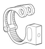
Wind the arm around the handlebar then close. If a plastic shim is used, rotate it to the correct position.
