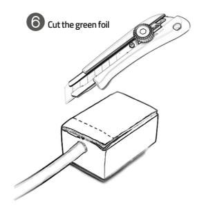
Cut a small section of the green adhesive backing foil as shown.
