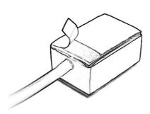
Remove the smaller piece of the green plastic foil. Keep the larger piece on the mounting tape.
