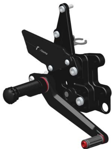
PER167-DX (Comandi arretrati lato DX completi) B (Complete RH rear set control kit)
