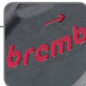
Logo Brembo lavorato in bassorilievo dipinto a mano. Low-relief machined Brembo logo. Hand painted finishing.
